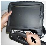
A) Insert the 'knobbed' end of the metal bar into the hole on the <u>left</u> of the case, as pictured here.
